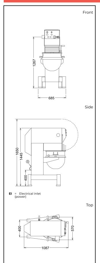
Electric 220-240/380-415 V/3 ph/50 Supply voltage: Electrical power, max: 1.54 kW **Total Watts:** 1.54 kW Capacity: ISO 9001; ISO 14001 kg/ Performance (up to): Cycle Capacity: 60 litres Key Information: External dimensions, 685 mm Width: External dimensions, 1087 mm Depth: External dimensions, Height: 1445 mm **Shipping weight:** 337 kg
